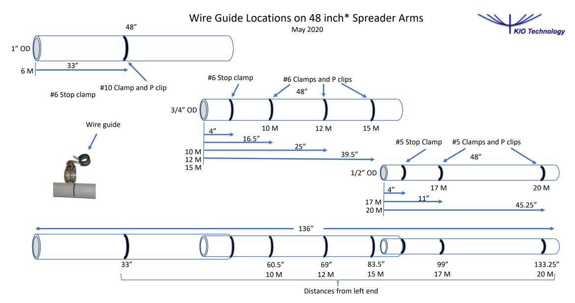
\*Replacement spreader arm sections from Max Gain Systems are 46.5 inches long instead of the standard 48 inches. So to compensate for this, the 4 inches telescoped lengths of the medium and small spreader sections should be reduced to 2.5 inches. This increases the splitting force on the ends of the large and the medium spreader sections and this splitting force can be offset by use of a clamp on the end as well as the stop clamp.
