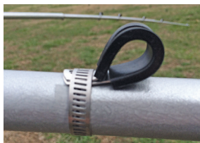
Figure 21 — The Adel clip and hose clamp combination for attaching wires is simple but effective.
